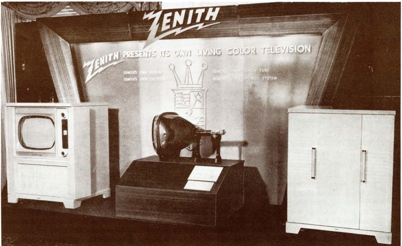
Color TV research and development by Zenith and Rauland provided the first 21-inch rectangular 3-gun color tube in 1954.
