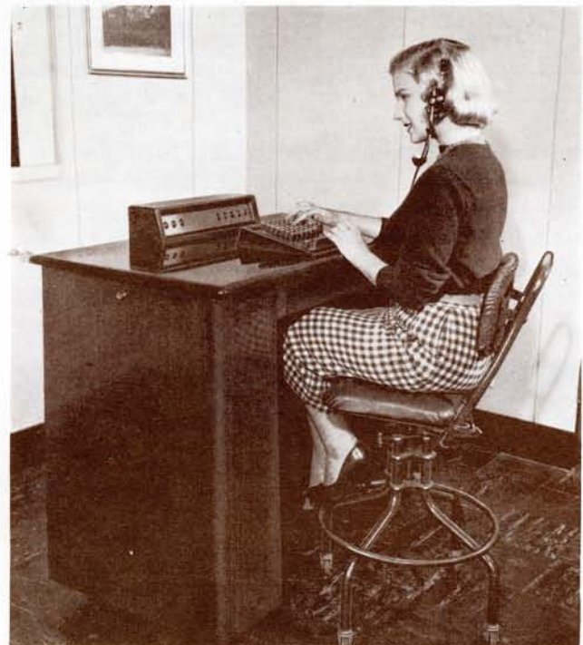
A "magic brain" Phonevision computer supplies proper decoding information to any subscriber requesting it by 'phone.
