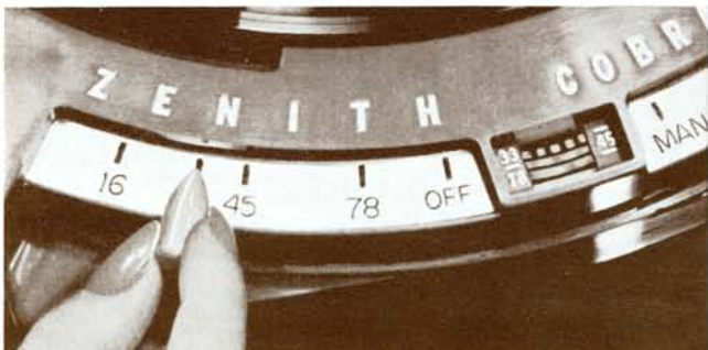
Among Zenith high fidelity advances are the speed control continuously variable from 10 to 85 rpm and the stroboscope indicator. Without them true high fidelity is impossible.
