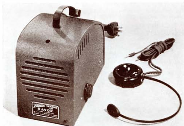
Designed for home and office use, the Ravox hearing aid operated on house current.
