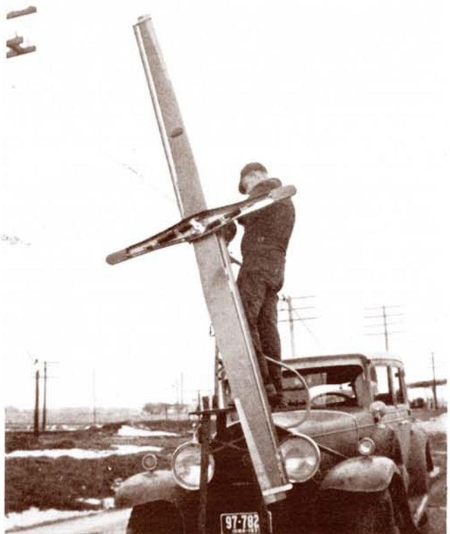
Early Wincharger development work used on automobile instead of wind tunnels for testing.
