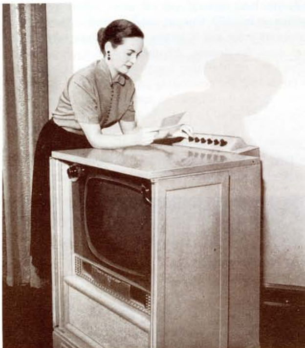
The Phonevision subscriber gets clear pictures and sound by properly adjusting the decoder mechanism on the TV set.
