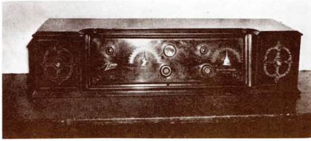
In 1926, the first commercially produced set to operate on AC household current came from Zenith. It freed radio of cumbersome batteries.
